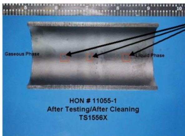
Figure 3 – 30 Day Sour Autoclave Test Conditions and As-Tested Sample
