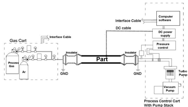
Figure 1: Diagram of Process Set-up [8].
