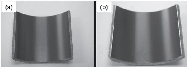
Figure 6: (a) DLC-Si coated internal surface of 304SS tube after 19hrs exposure to a 15% hydrochloric acid solution, (b) DLC-Si coated internal surface of 304SS tube after 19 hours exposure in 10% sodium chloride solution at 70°C.
